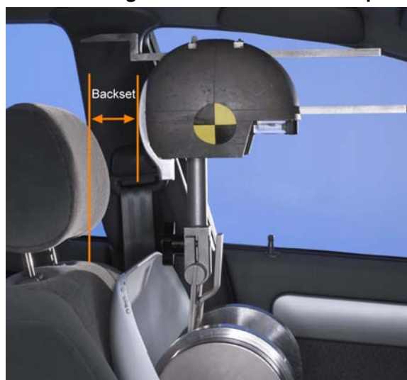
Figure 9 Measuring Backset for BioRID Set-up
