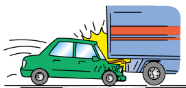
② Collisions where the impact is gradual as when driving under the load space of a truck.
