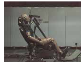
Neck injury protection for rear-end collision
