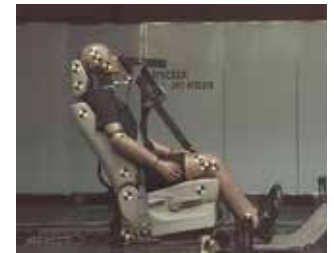
Neck injury protection for rear-end collision
