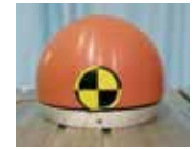
Adult head impactor (165mm in diameter and 4.5kg in mass) Child head impactor (165mm in diameter and 3.5kg in mass)
