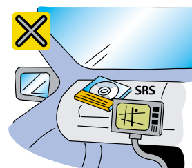
Do not place objects on top or in front of the instrument panel.
