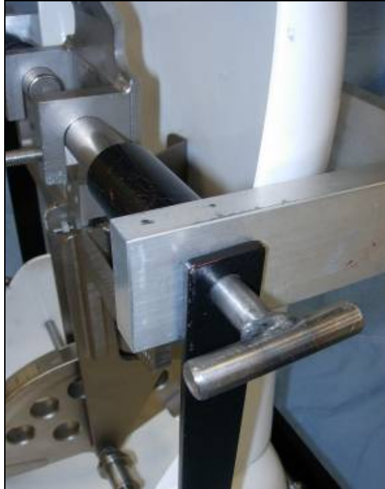
Figure 5. Weight hanger support pins inserted through weight hanger guide bars.
