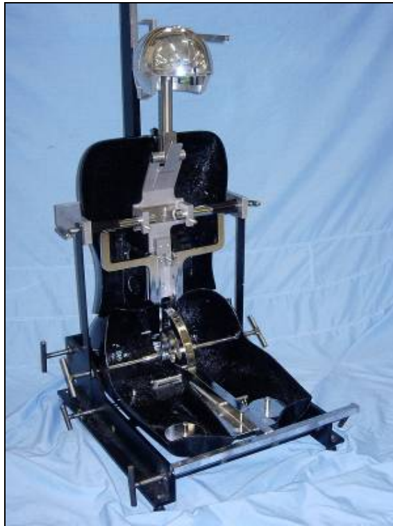
Figure 7. H-PM in calibration jig with H-point to arm supports
