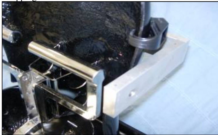
Figure 4. H-PM back pan held by retaining strap
