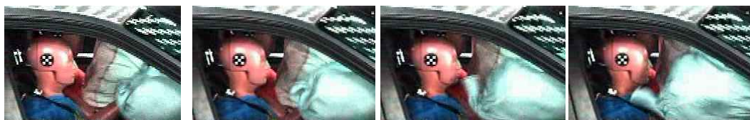
Example of an airbag flap unfolding within the Head Zone.
