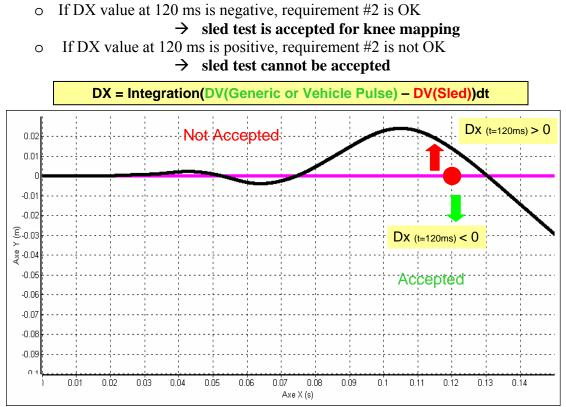
Sample picture shows a sled test that cannot be accepted as DX is positive @ 120 ms
