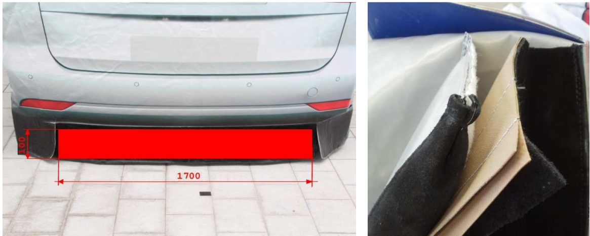
Figure A.2.2-1: Left, Front view of the EVT with the location of the lower radar absorption mat. Right, different layers of absorption mat
