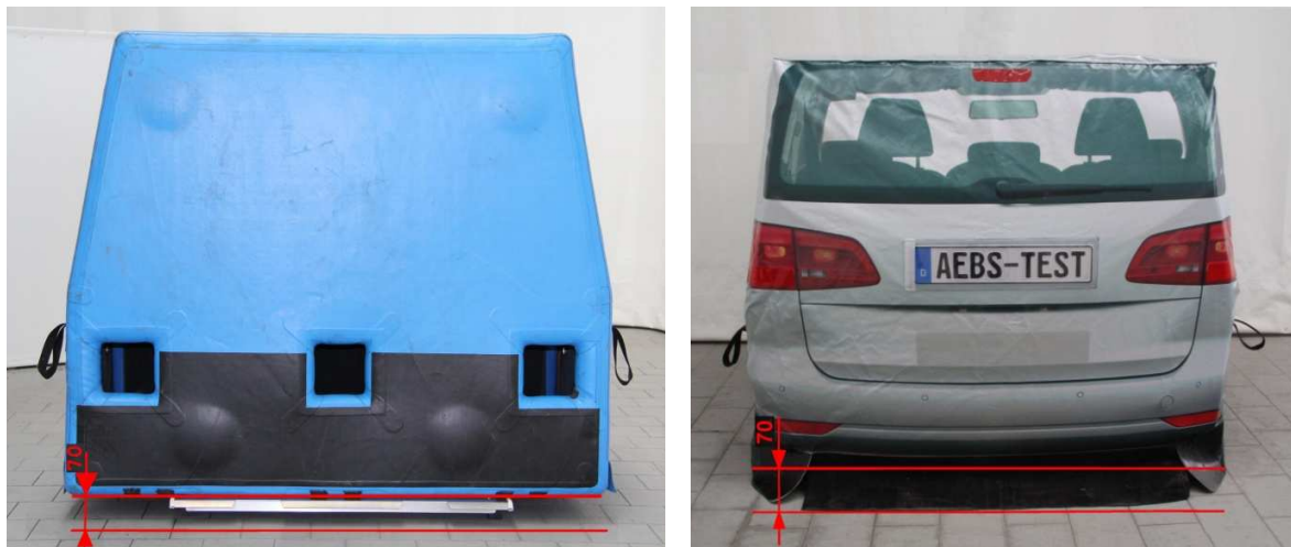
Figure A.3-1: Front view of the EVT showing the ground clearance
