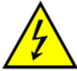
Figure 1 Marking of high voltage equipment
