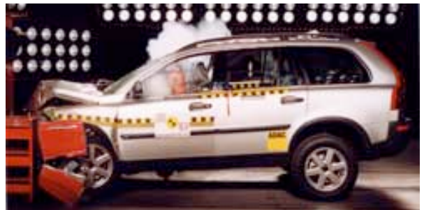
Offset crash test at 64km/h
