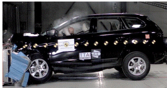
Offset crash test at 64km/h
