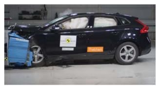
Frontal offset test at 64 km/h (Source: Euro NCAP)
