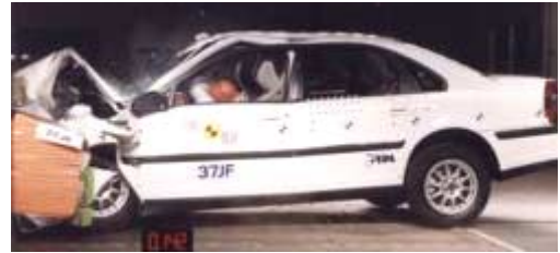
Offset crash test at 64km/h
