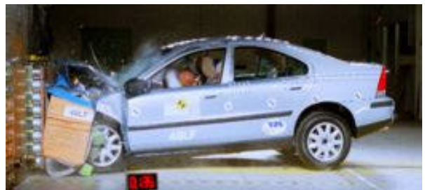
Offset crash test at 64km/h
