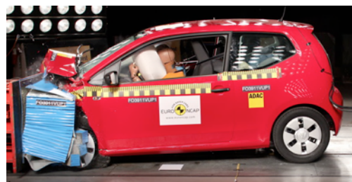
Offset crash test at 64km/h
