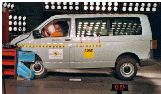
Offset crash test at 64km/h
