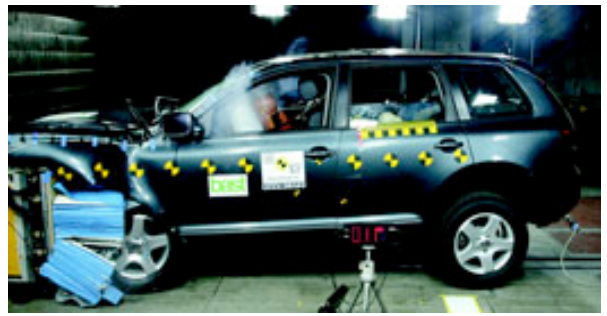
Offset crash test at 64km/h
