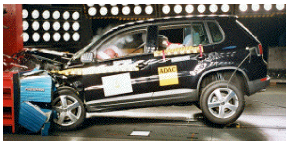
Offset crash test at 64km/h
