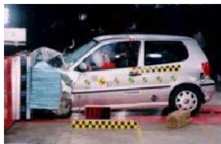
Offset crash test at 64km/h
