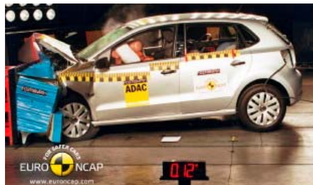
Frontal offset test at 64 km/h (Euro NCAP 2009)
