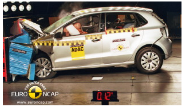
Offset crash test at 64km/h
