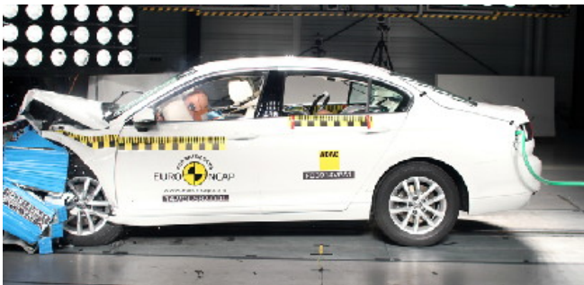
Frontal offset test at 64km/h
