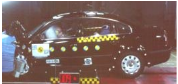
Offset crash test at 64km/h
