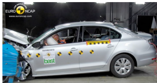
Offset crash test at 64km/h
