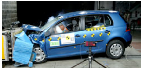
Offset crash test at 64km/h
