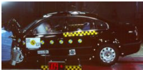
Offset crash test at 64km/h
