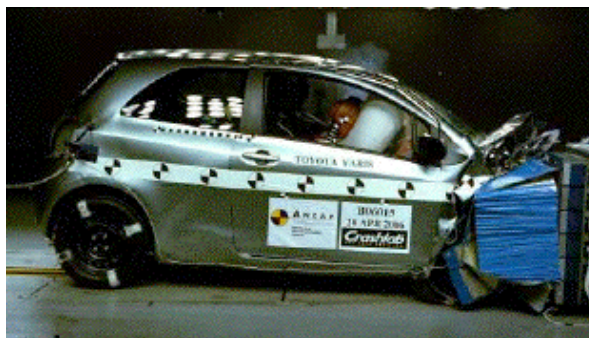
Offset crash test at 64km/h
