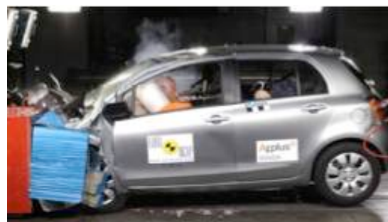
Offset crash test at 64km/h
