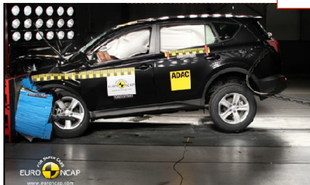
Frontal offset test at 64km/h
