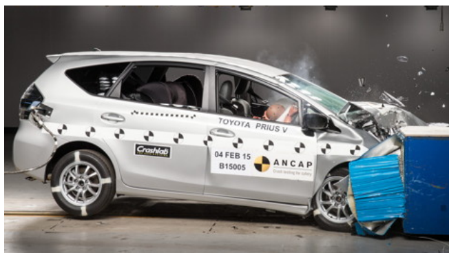
Frontal offset test at 64km/h
