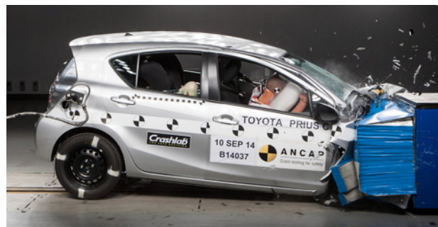
Frontal offset test at 64 km/h
