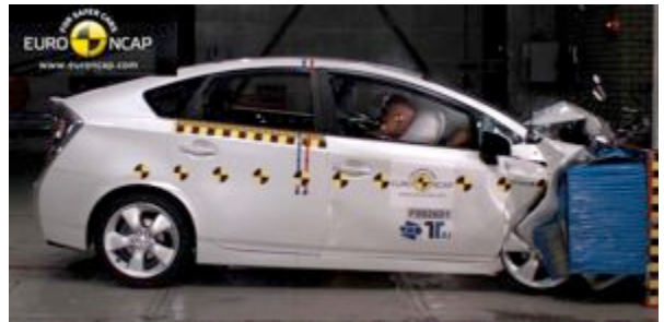
Offset crash test at 64km/h
