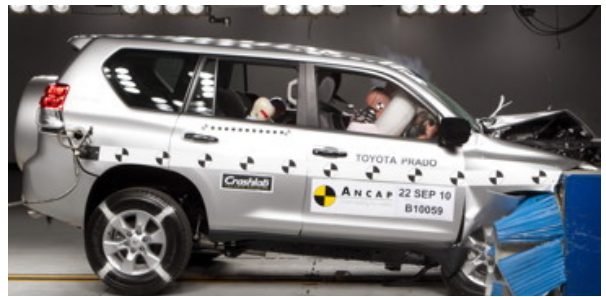
Offset crash test at 64km/h
