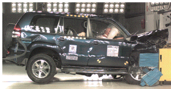
Offset crash test at 64km/h
