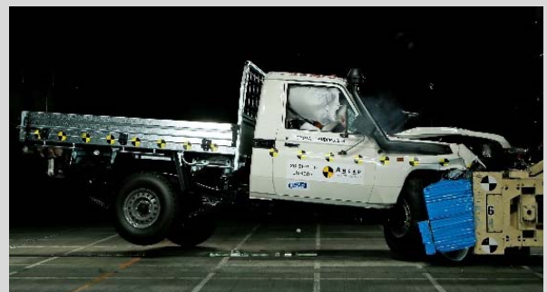
Frontal offset test at 64km/h
