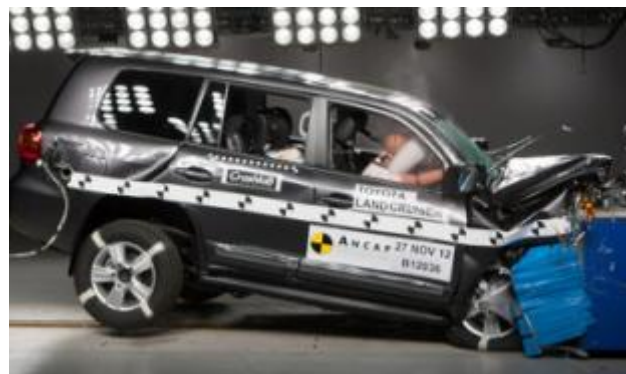
Frontal offset test at 64 km/h
