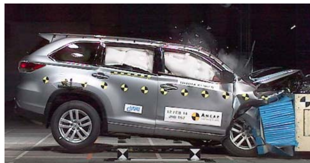
Frontal offset test at 64 km/h
