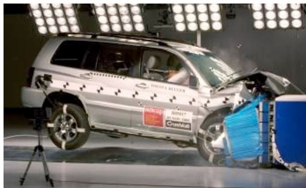
Offset test at 64km/h
