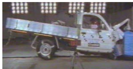
Offset crash test at 64km/h
