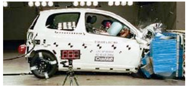
Offset crash test at 64km/h
