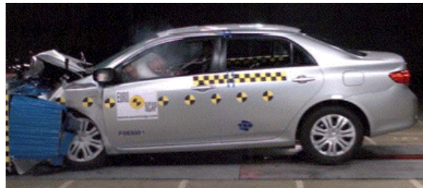
Offset crash test at 64km/h
