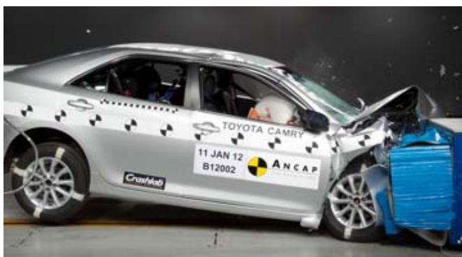
Frontal offset test at 64km/h
