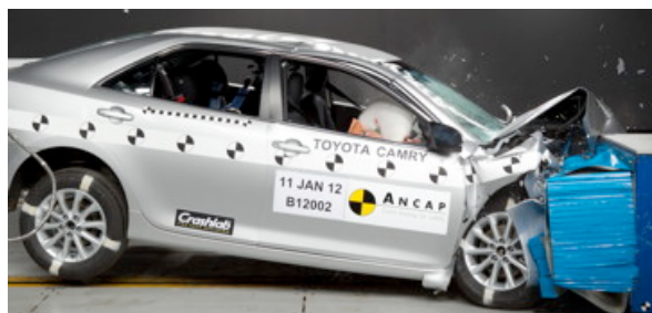
Offset crash test at 64km/h
