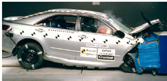
Offset crash test at 64km/h
