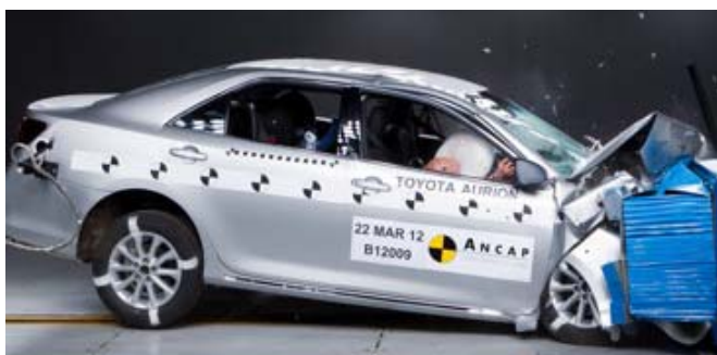
Frontal offset test at 64km/h
