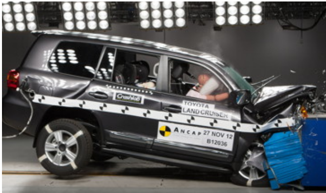
Frontal offset test at 64km/h
