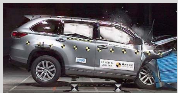
Frontal offset test at 64km/h
