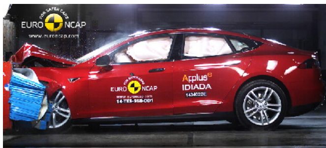
Frontal offset test at 64km/h
