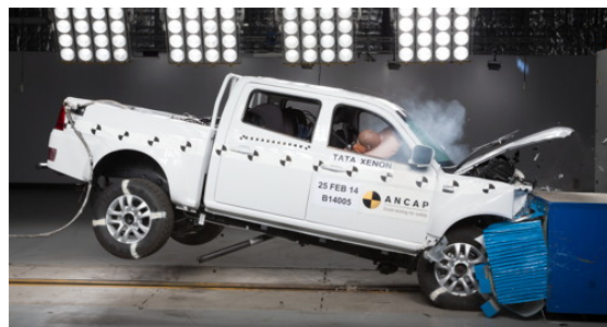
Frontal offset test at 64 km/h
