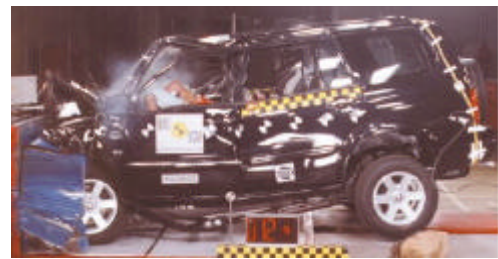
Offset crash test at 64km/h
