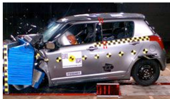
Offset crash test at 64km/h
