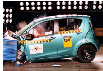
Offset crash test at 64km/h
